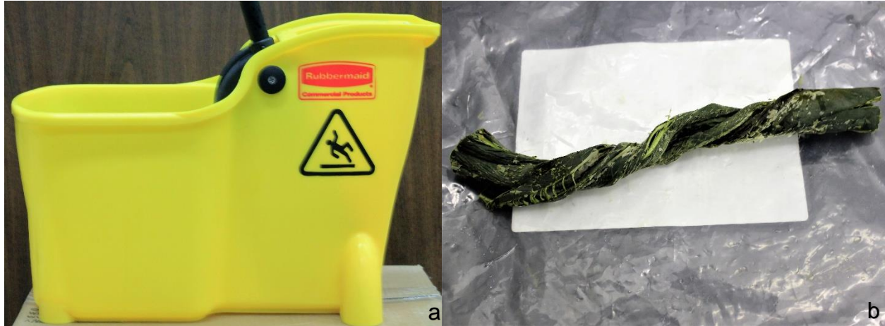
Figure 4. Picture of Blue Agave leaf juice extraction methods. (a) Initially, juice from Blue Agave leaves was obtained with a makeshift juicer; comprised of a mop wringer and bucket. This worked, but not as well as simply wringing the thawed leaves out by hand. (b) Hand wringing the leaves was the method used for the fermentations in this work; the leaf on the right was processed by the hand method.
