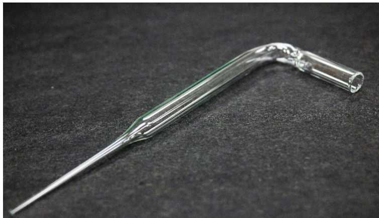
Figure 9. Picture of plate spreader. CFU plates were made by spreading samples on solid growth medium. This spreader was made by heating a Pasteur Pipette with a Bunsen Burner until soft enough to bend with forceps and an insulated glove. They were sterilized by autoclave and sealed until use.
