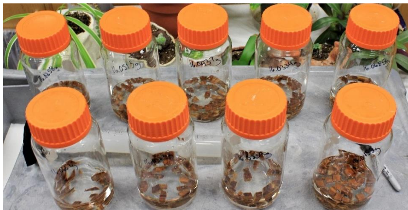
Figure 5. Picture of cocoa pod husk pieces in water. The cocoa pod husk (CPH) had been thawed, weighed, divided and suspended in nanopure water. Once autoclaved and cooled, the CPH was inoculated with one of two strains of yeast, or used as a control with no cells added.
